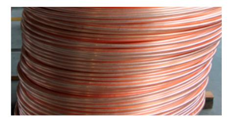
Copper wire rod is used for the production of the electrical products: wires, tires, rods, etc.
